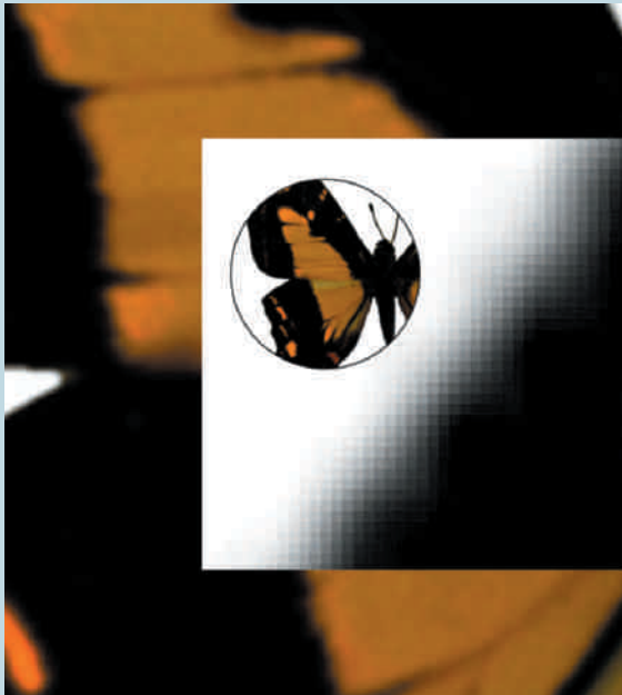
↑ 11-6 Enlarging a raster image on a monitor will reveal its pixel structure.
